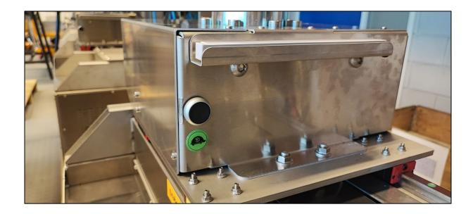
This button adjusts the rotation speed of the turntable according to the mechanic's preferences. When the button is pushed inwards, the 'slow start' function remains constant. When the button is released, the machine starts with general slow start and continues to normal speed.
